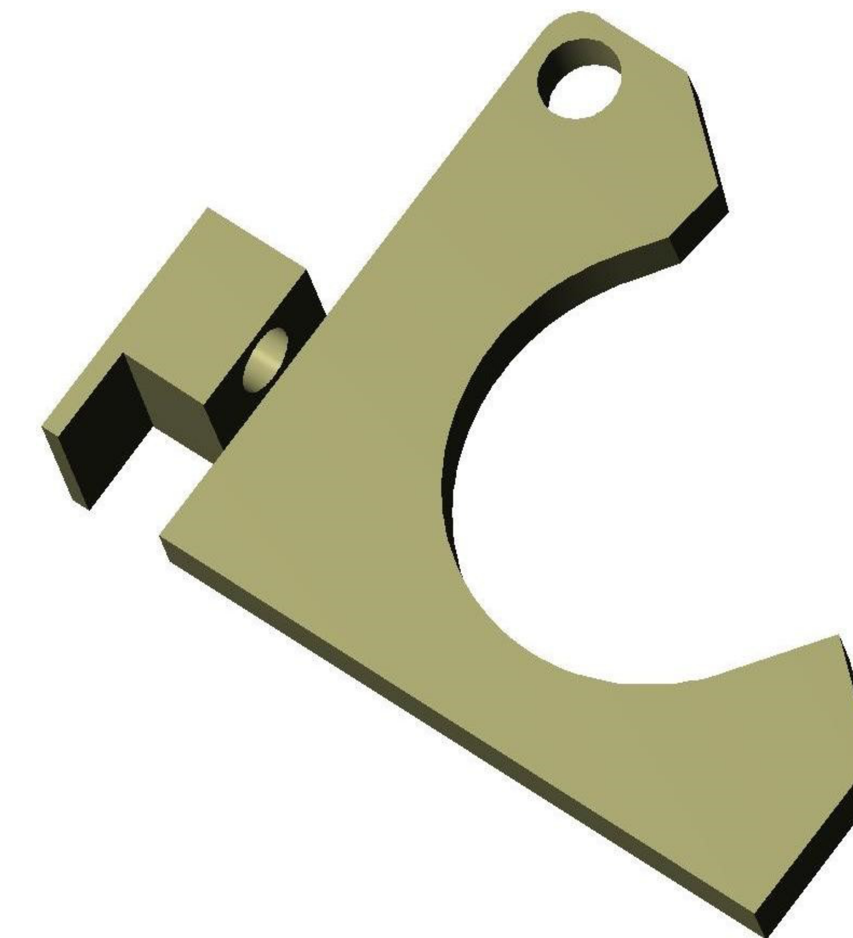
Improved dosing block locking disc (small) 02-390-188
